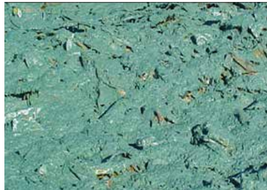
A polysaccharide tackifier increases the surface bond to debris, including plastic and other slick-surface materials, ultimately lowering blowing debris and trapping odors
